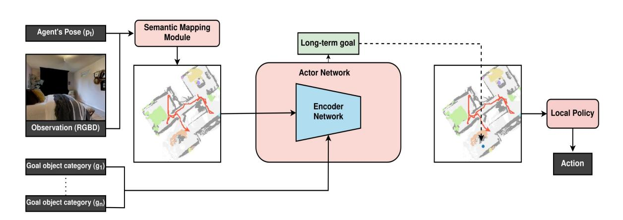
When a long-term goal is provided by the actor-critic network, the local policy module uses the Fast Marching Method(FMM) to guide the robot to this region by utilizing the obstacle channel of the generated semantic map.
